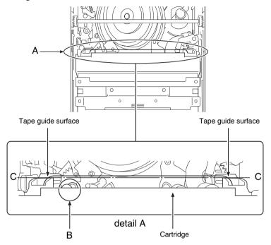
The Initial Position of the Threading Mechanism
